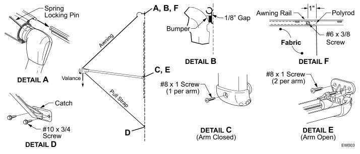
Figure 5. Mounting the Awning.
