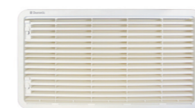
LS300 vent and frame cut out required W490 mm x H249 mm. Each vent has open area of 667 cm 2
