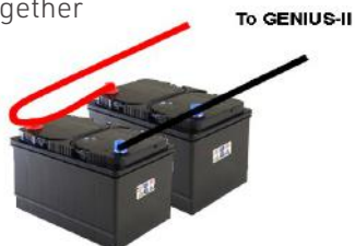
Figure 4: Recommended wiring for connecting batteries in parallel
