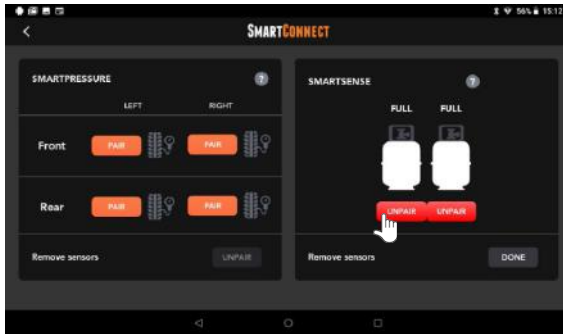
Figure 14: Unpairing the SmartSense gas bottle level sensor
