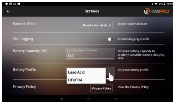
Figure 9: Configuring a new battery from the JHub App settings.
