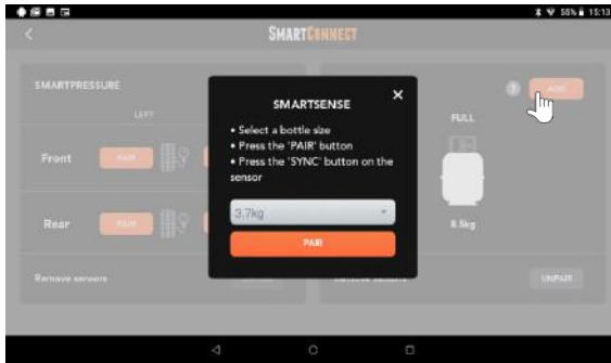
Figure 10: Adding a new SmartSense gas bottle level sensor
