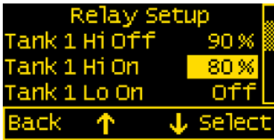
Relay Setup Screen with Relay Normally = On (Closed)
