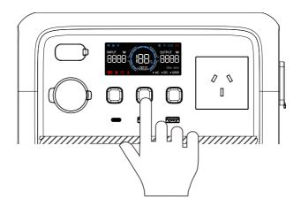
• Power ON: Press and hold the POWER Button for about 2 seconds, the button lights up indicating that the AC2P is now on standby.
