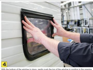
With the bottom of the window in place, gently push the top of the window in position in the opening. Insert screws into pre-drilled holes in main frame, Do Not Tighten screws until all screws have been inserted and window is in position. Once in position, fully tighten all screws in opposite sequence until all screws have been secured.
