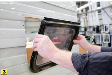
Fill cladding seams with silicone then crush final 10mm. Position window in opening on the wall of the van where it is going to be permanently installed. Do this from the outside of the van. Bottom of the window to go in first - to clear thumb locks.
