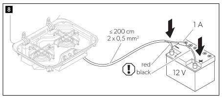
► Add a 1 A fuse in the plus line near the battery.
