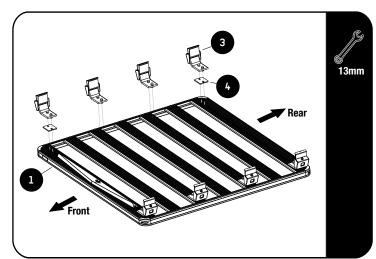
Loosely assemble the Legs & Spacers (Items 1, 3 & 4) as shown, slats indicated in 2.2 using M8 Flat Washers and M8 Nyloc Nuts included in the Leg sets.
