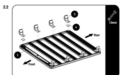
Loosely assemble the Legs & Spacers (Items 1, 3 & 4) as shown, slats indicated in 2.2 using M8 Flat Washers and M8 Nyloc Nuts included in the Leg sets.
