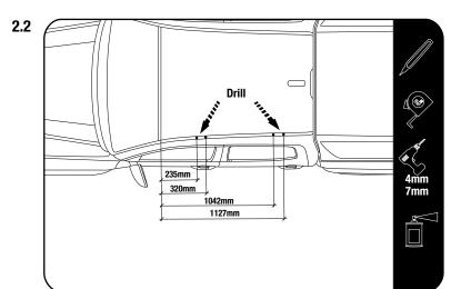
Starting at the top edge of the windscreen measure along the ditch towards the rear of the vehicle. Mark the hole centre's in the ditch as shown.
