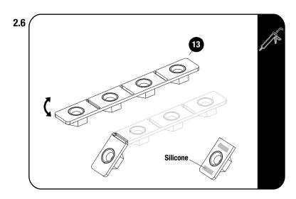
Twist the nut plates (Item 13) free from each other and apply silicone before the fitment in step 2.7.
