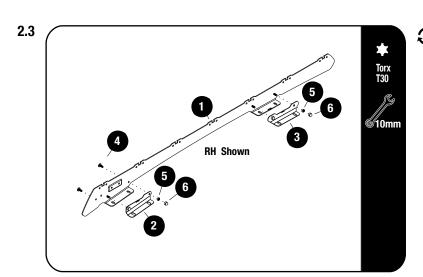
Secure the Stiffener Plates (Items 2 & 3) to the Foot Rails (Item 1), using M6x16 Flange Button Heads & M6 Nyloc Nuts (Items 4 & 5). Fully tighten.
