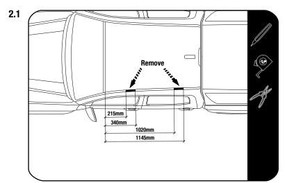
Starting at the top edge of the windscreen as shown, measure along the ditch moulding towards the rear of the vehicle. Mark the ditch moulding at the following distances.
