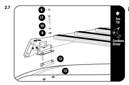
Place silicone over the 8 holes drilled in 2.2.
