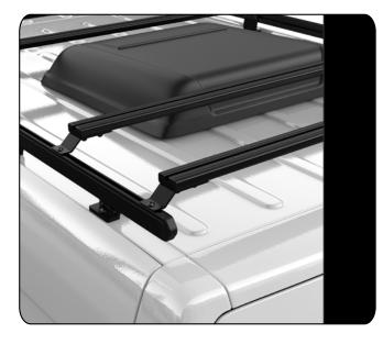
If a roof A/C is fitted to the vehicle space the slats around the A/C at 202mm increments on shorter lengths and 404mm on the longer lengths
