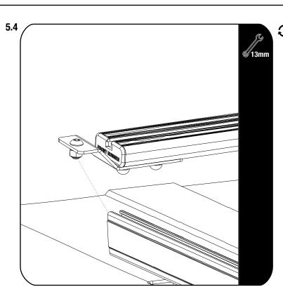
The Slat Z brackets can be inverted as shown if you wish to have the rack lower on your vehicle.
