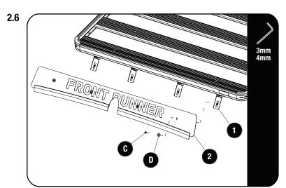
Remove the M5x16 Countersink Screws and M5 Finishing Washers from the Brackets. Loosley secure the Wind Fairing to the Brackets using the M5x16 Countersink Screws and M5 Finishing Washers. Adjust the Bracket angle and position as required.
