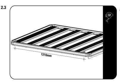
Adjust the M8 Eyenuts ( Item 3 ) to measure 1210mm centre to centre as shown. Fully tighten.
