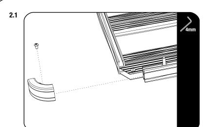
Loosen and remove the corner of the Rack as shown
