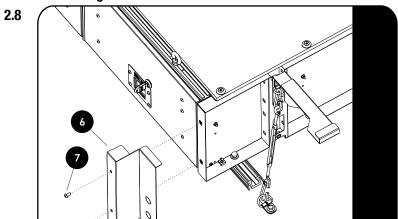
Secure the Front Faces (Item 5 & 6) to the Cage Nuts in the Drawer System (SSDR010) using M6 x 12 Button Heads (Item 7) as shown.
