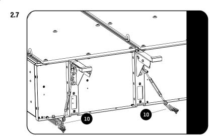
Secure the D-Rings supplied with SSDR010/SSW0008 using the holes you drilled in Step 2.1.
