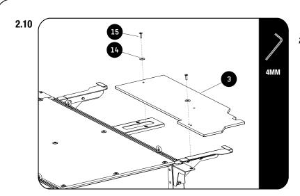
Fit the LH & RH Rear Decks (Items 2 & 3) with M6 x 30 Countersink Screws and M6 Finishing Washers (Items 14 & 15) as shown.
