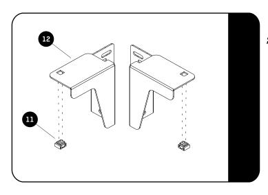
Before you start to fit the wing brackets to the Drawer, clip the M6 Cage Nuts (Item 11) into the Rear Corner Wings (Item 12 & 13) supplied with SSDS602.
