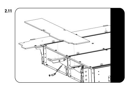
Fit the Side Decks (Items 1 & 4) to the Drawer by sliding it into the C-Clips.
