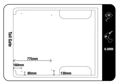
Using the measurements shown, measure and mark the positions of the holes you need to drill. Do this on both left and right side of the loadbed.
