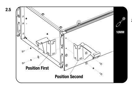
When fitting the Rear Corner Wing Brackets (Item 12 & 13) take note of the position. Item 12 & 13 needs to be placed on the Drawer first, followed by the corner wing supplied with SSWS001.
