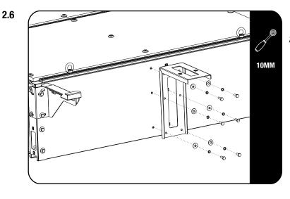
The rear support bracket is also part of SSWS001. Fit and secure with the fasteners supplied with SSWS001 as shown.
