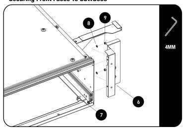
Secure the Front Faces (Item 5 & 6) to the Wolf Box System (SSW0008) using M6 x 12 button Heads, M6 x 12 x 1SS Flat Washers and M6 Nyloc Nuts (Item 7, 8 & 9) as shown.
