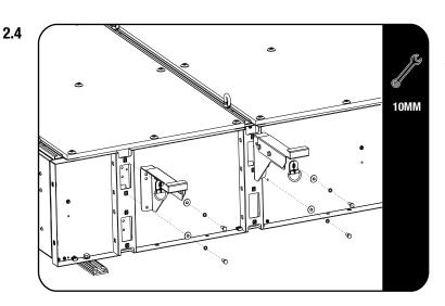
Refer to the SSWS001 fitting instruction to assemble the Wing Brackets before you start to fit them to the Drawer.
