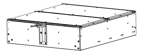
( **G** ) Reffering to the diagram below, mark out the vehicle's load bay and drill a 6.5mm on each of your four markings.
