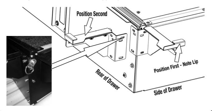
( **D** ) Secure the front and rear of the Drawer System to the vehicle using the 37 mm C-hooks and Turnbuckles (Items 2 & 36) as shown below. Ensure Drawer remains centered, left to right, and 45 mm in from the edge of the load bay (Refer to Step 3A).
