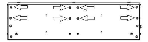
(F) Using six M6 x 20 Hex Hex Bolts, six M6 Spring Washers and six M6 x 19 Flat Washers removed in Step 2E, secure the Rear Support (Item 23) to the back of the Drawer System as shown.
