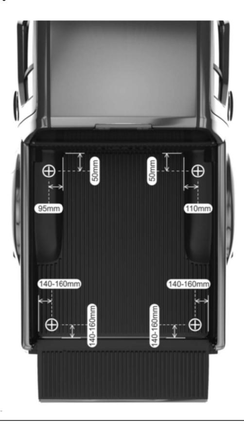
( H ) Using the components received with SSDS501, secure the four D-ring's (Item 32) to the inside of the Load Bay. You will be bolting through each of the holes drilled in Step 2G using a M6 x 25 Hex Bolt, two M6 x 19 Flat Washers and a M6 Nyloc Nut per D-ring (Items 33, 34, 35) as shown.
