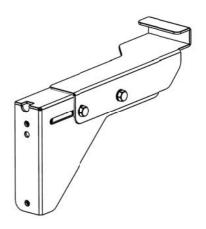
( **B** ) Using Step 2A as a guide, loosely assemble the Corner Wings (Items 24, 25, 26) as shown.
