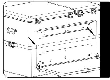
Using the Ratchet Strap (Item 1) secure the table to the Fridge using the slots in the table as shown. Check table clearance before fully tightening.
