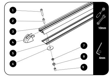
Fit and secure the tracks with a combination of Items 1/2, 6, 7, 8 & 9.
