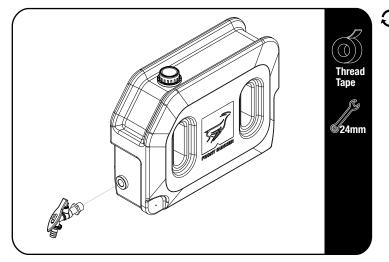
If you are fitting the tap apply thread tape to the thread of the tap.
