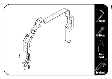
Apply anti-rust around all the holes. Place some silicone around each hole.
