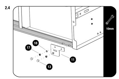
Slide both Stud Plates from 2.3 to either side of the extrusion, against the side of the Drawer. Secure the Mounting Plates (Item 11) to the Stud Plates using four M6 Flat Washers and four M6 Nyloc Nuts (Items 17 & 18).
