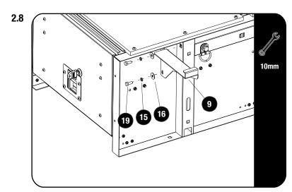
Secure the Right Front Wings (Item 9) to the Drawer System using four M6 x 16 Hex Bolts, four M6 Spring Washers and four M6 x 19 Flat Washers (Items 15, 16, 19) as shown.
