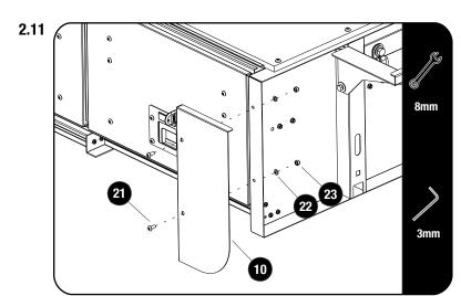
Secure the Left and Right Front Faces (Item 10) to the Drawer System using four M5 x 12 Button HeadBolts, four M5 Flat Washers and four M5 Nyloc Nuts (Items 21, 22, 23) as shown.
