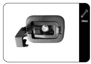
Loosen and remove the two tie down points located on the floor of the vehicle behind the rear passenger seats.
