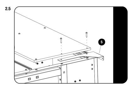
Loosen the nine Countersunk Bolts securing the Rear Deck to the Drawer System.
