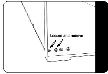
Working at the bottom right rear corner of the Drawer, use the Square Recess Bit (Item 24) provided and remove the two screws as indicated.
