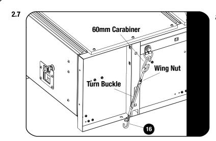
Secure the front of the Drawer System to the tie down points at the rear of the vehicle using two M6 Turn Buckles, two 60 mm Laser Cut Carabiners (supplied with SSDR005) and two 37 mm Laser Cut Carabiners (Item 20) as shown.
