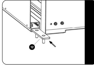
Pull the Drawer's backing plate and the attached aluminium extrusion away from the corner of the Drawer as shown.
