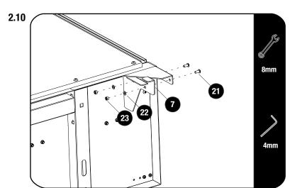
Secure the Left and Right Rear Wings (Item 6 & 7) to the Wing Brackets fitted in 2.6 using four M5 x12 Button Head Bolts, four M5 Flat Washers and four M5 Nyloc Nuts (Items 21, 22, 23) as shown.
