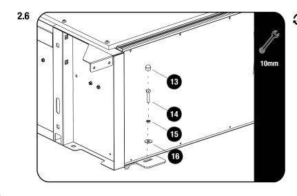
Place the Drawer System into the vehicle lining up the holes in the Mounting Plates from 2.4 with the threaded mounting points in the vehicle's floor from 2.1.
