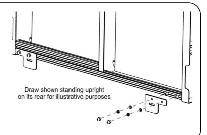
Loosen the nine Countersunk Bolts securing the Rear Deck to the Drawer System. Lift the Deck and place the Left and Right Hand Rear Wing Brackets (Items 15 & 16) in position between the Deck and Drawer System as shown. Secure the Deck back to the Drawer System, "sandwiching" the Wing Brackets between the Deck and Drawer System.
