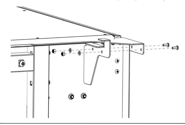
( **E** ) Secure the Left and Right Front Faces (Item 14) to the Drawer System using four M5 x 12 Button Head Bolts, four M5 Flat Washers and four M5 Nyloc Nuts (Items 25, 26, 27) as shown.
