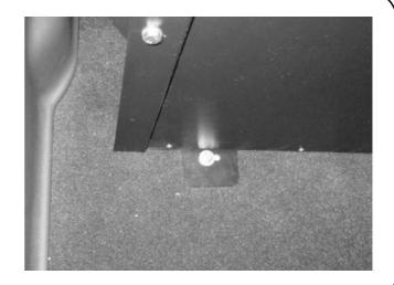
( **B** ) Secure the front of the Drawer System to the tie down points at the front of the vehicle using two M6 Turn Buckles, two 60 mm C-Hooks and two 37 mm C-Hooks (Items 2, 6, 30) as shown.
