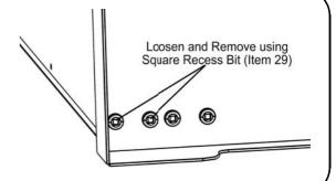
Pull the Drawer's backing plate and the attached aluminium extrusion away from the corner of the Drawer as shown. Slide the two Stud Plates (Item 18) in to the extrusion as illustrated.
