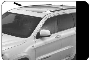
Remove the factory roof rails as shown.
