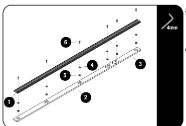
Locate the mounting points on the vehicles roof and secure the Tracks, Front Spacers and Rear Spacers (Items 1, 2 & 3) using M6 x 20 Button Head Bolts and M8 x 16 x 1.6 Flat Washers or M8 x 19 x 2 Flat Washers (Items 4, 5 & 6).
