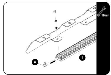
Secure the Foot Rail (FAJG001) to the Track (Item 1) using the fasteners supplied with RRAC976, Stud Plates (A), M6 x 12 x 1 Flat Washers and M6 Nyloc Nuts.
