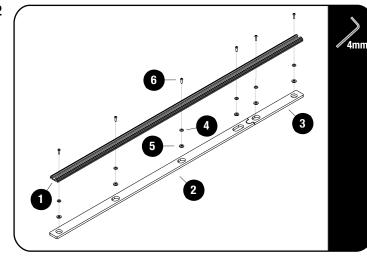
Locate the mounting points on the vehicles roof and secure the Tracks, Front Spacers and Rear Spacers (Items 1, 2 & 3) using M6 x 20 Button Head Bolts and M8 x 16 x 1.6 Flat Washers or M8 x 19 x 2 Flat Washers (Items 4 5 & 6) (Items 4, 5 & 6).
