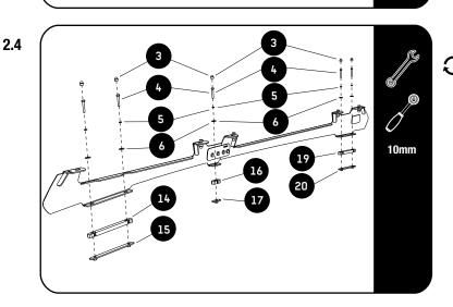
Place the assembled foot rail onto the spacers and secure with items 4, 5 and 6 using the nut plates, item 15,17 and 20 on the inside of the roof. Place a bead of sealant on the nut plates top side before securing them. See diagram 2.5.
