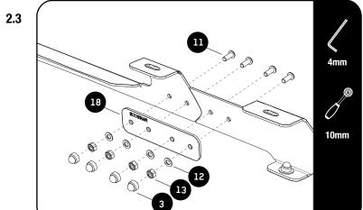
Join the two sections of the foot rails with the supplied splice plate (Item 18). Fasten as shown with items 11, 12 and 13. Fit item 3 over each nut after fastening the bolts.
