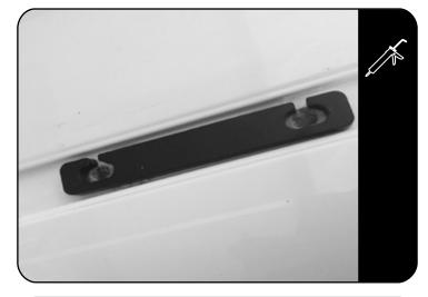
Place a bead of sealant in and over each hole in the roof, then place a spacer over each hole.
