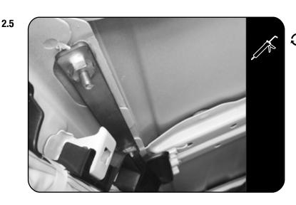
Nut plate shown on the inner side of the roof.
