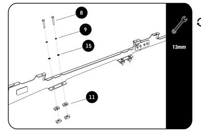
Secure the Foot Rail using M8 x 40
