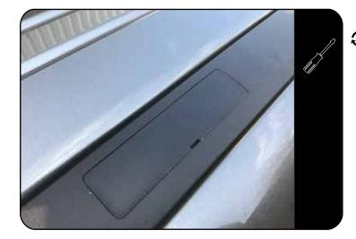
Before starting the fitment you need to remove the front, middle and rear Ditch Covers from the vehicle's roof using a suitable flat screw driver.
