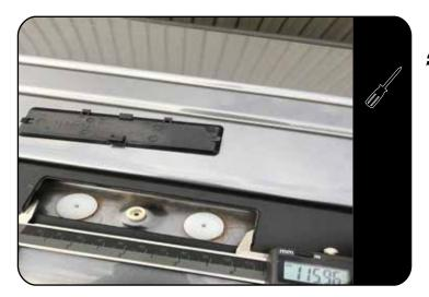
Remove the plastic two inserts with a Philips screw driver.
