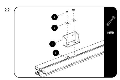
Loosely fit a Leg Mount (Item 3) to each of T-Bolts using M8 x 19 x 2 Flat Washers and M8 Nyloc Nuts (Items 5 & 7).
