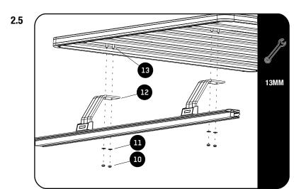
Loosely fit your Slimline II Rack by using M8 x 25 Hex Bolts, M8 x 16 x 1.6SS Flat Washers and M8 Nylocs (Items 10, 11, 13) as shown.
