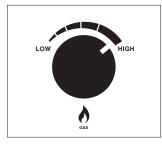
To increase Water Temperature turn GAS Control to HIGH and allow temperature to stabilise.
