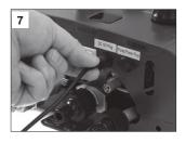
Check that the switch on the unit is in "OFF" position and then connect the power cable for the 12VDC Power Supply. Connect the male cigarette fitting to a suitable DC power source.
