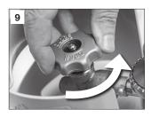
Turn the gas cylinder on in an anti-clockwise direction one (1) full turn, then check all LP Gas connections for leaks with a solution of soapy water (do not use a flame). If a leak is detected turn the cylinder valve off, allow any residual gas to disperse, retighten all connections then retest.
