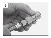
Attach the FEMALE section of the Quick Connect Gas Fitting to the Hose & Regulator assembly, ensuring that Thread Tape is used.
