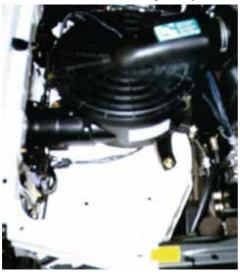
3. Place and bolt the tray into the Engine Bay, using the 2 x M6 Counter sunk bolts, washer and nuts on the underside.
