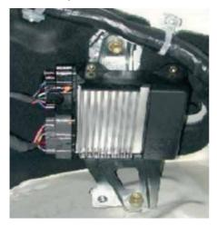
3. Refit diesel computer to supplied computer bracket using the 3 original screws.
