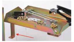
5. Install an M6 bolt through front of tray, secure with nut and body washer under guard.
