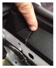
Using top mount Anchor Bracket mark hole centre and drill two 9mm holes. Using a Rivet Nut gun install 2 x Nutserts (Supplied) in to top of guard. Insert M6 bolts and secure anchor bracket to top of guard.
