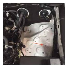
4. Line up other holes and using M6 bolt with nut and body washer secure rear arm closest to engine.
