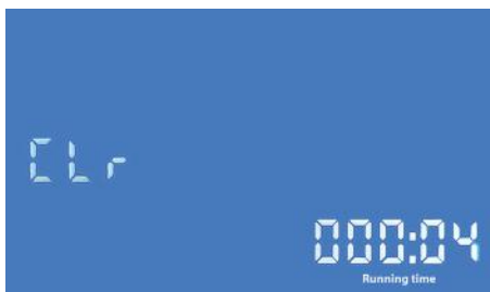
Figure 11: Clear the running time interface
