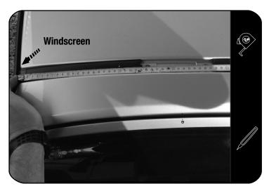
Starting at the front windscreen as shown, measure along the Ditch Moulding towards the rear of the vehicle. Mark the Ditch Moulding at the following distances 240mm and 375mm.
