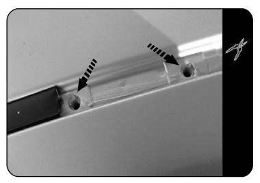
Using a pair of tin snips, cut the Ditch Moulding on each of your marks and remove the small strips of Ditch Moulding between markings 1-2 and 3-4.
