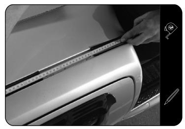
Still measuring from the front windscreen mark the Ditch Moulding at the following distances 1245 mm and 1410 mm.
