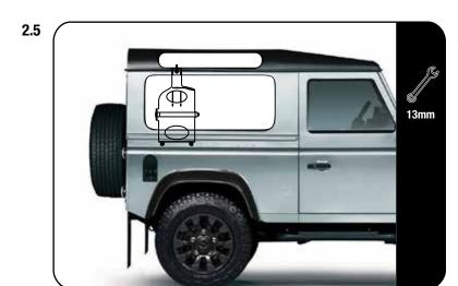
Fully tighten the gutter clamp bracket that was loosened in 2.1
