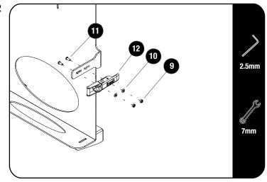
If needed adjust the Latch (Item 12) using two M4 x 10 Button head, two M4 Flat Washers and two M4 Nyloc Nuts (Items 9,11 & 11) so that it accomodates your Jerry Can before fully tightening.
