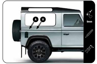
Place the Vertical Jerry Can Holder (Item 8) on the side of the vehicle so that it fits over the top gutter and lines up with the two rivets (Item A) on the vehicle body as shown in 2.3.
