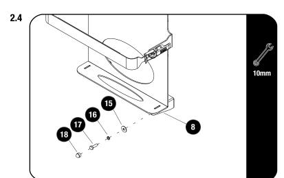
Mount the Vertical Jerry Can Holder (Item 8) to the vehicle using two M6 x 20 Hex Bolts, two M6 Spring Washers and two M6 Flat Washers (Items 15,16 & 17).
