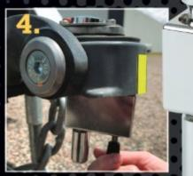
With the key barrel facing the ground, slide up the locking case as far as it will go. Insert the key and lock closed.
