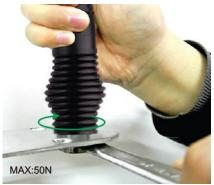
3. Remove the cap from the top of the spring base and install the fiberglass extension pole on to the base by turning in a clockwise direction and secure in palce with the grub screw (using the hex key provied). Hand tighten only MAX. 15N.
