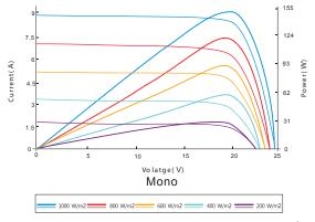
Excellent performance under weak light conditions: at an irradiation intensity of  $800W/m^2$  (AM 1.5, 25°C), 95.5% or higher of the STC efficiency(1000W/m<sup>2</sup>) is achieved.
