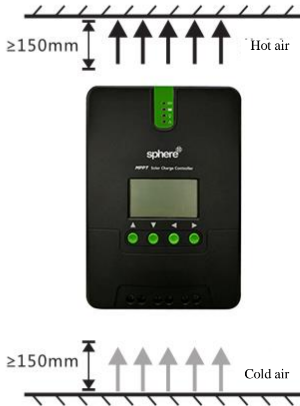
Fig. 2.1 Installation and heat dissipation
