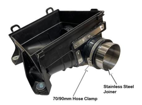
Re-install the air cleaner base and fasten using the standard mounting bolts.
