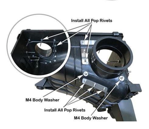
With the air entry hose, pop rivets and hose support plates correctly installed, secure all the pop rivets using a pop rivet gun.
