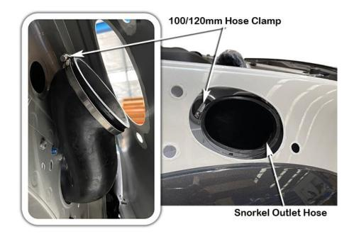
When correctly aligned, fasten the snorkel body to the guard panel with body washers (Item 8) and nyloc nuts (Item 9).
