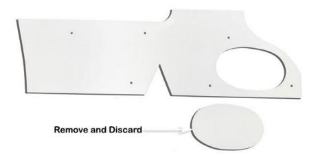
Align the guard panel template (Item 21) to the upper and rear edges of the right hand guard panel as shown.
