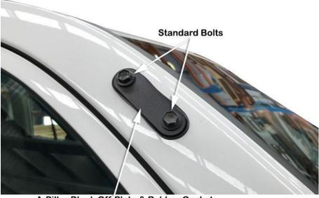
A-Pillar Blank Off Plate & Rubber Gasket
