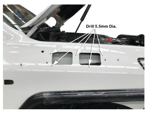
The front factory captive mounting nut assembly must be removed.
