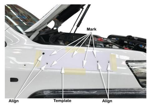
Drill a pilot hole for each of the marked hole positions, drill the five hole positions to 5.5mm diameter using a 5.5mm drill bit.
