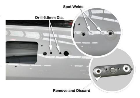
Remove and discard the perforated section of the guard panel template (item 21) as shown.
