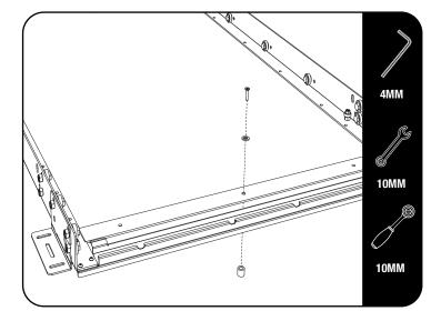
Place the frame back onto the load bed and secure using the fasteners and spacers supplied. The spacers (Item 5) are to be used when the mounting points are in a "dip" and not on a raised section by placing it over the rivnut so that the frame rests on the spacer.
