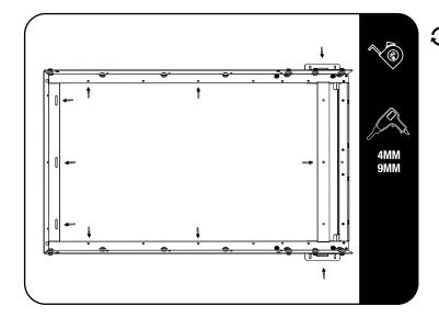
Make sure you have closed the load bed tail gate to ensure that it does not make contact with the frame. Once you are satisfied with the positioning of the frame, mark the position of all the mounting points as indicated by the arrows onto the load bed.
