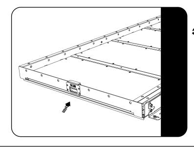
Refer to Step 2.2, refit the tray and stoppers. Once refitted check that the push to close latch engages fully and that the slide is secure.
