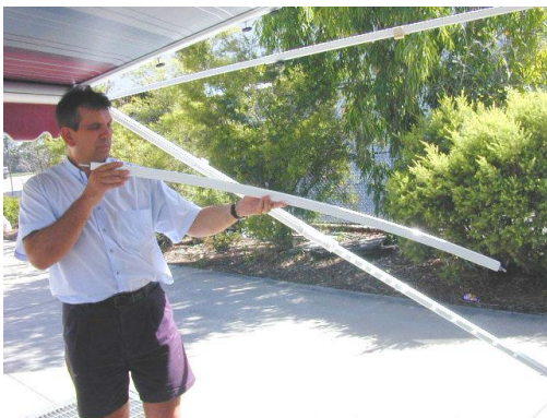
Rafter retracted for travel, undo the knob to extend out.
