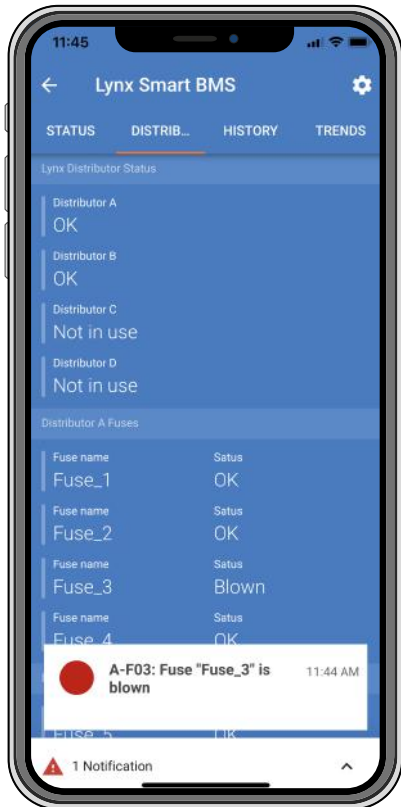
Examples of a fuse alarm on the VictronConnect App and on a GX device
