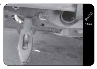
Run the tap assembly towards the rear left of the bumper. Secure the locking tap to the bumper. Using a M8 x 25 Hex Bolt, two M8 Flat Washers, and a M8 Nyloc Nut (Item 7, 8 & 10).
