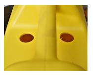
The holes are drilled into the jerry can using a step drill bit.
