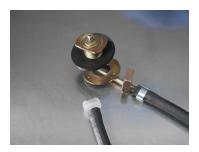
The breather tube fits onto the straw and is clamped down with an ear clamp.
