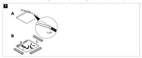
8. Fit the reinforcing rails (B).
