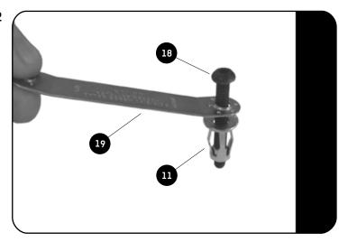
Insert the M6 Button Head Bolt (Item 18)into the one side of the Installer Wrench (Item 19). Loosely fit a Jack Nut (Item 11) to the Button Head Bolt as shown.
