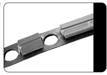
Using a 22mm hole punch "recommended" or hole saw, punch/drill holes through the ditch molding on each of your markings.
