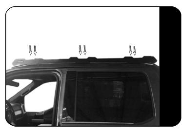
Using a flat screw driver and starting from the front of the vehicle, lift and remove the two ditch moldings running along either side of the roof.
