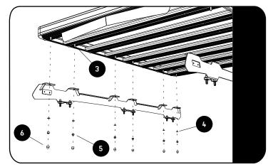
Fit your Roof Rack to the Foot Rails using M8 x 20 Hex Bolts, M8 x 16 x 1.6SS Flat Washers and M8 Nyloc Nuts (Items 3, 4 & 5).
