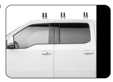
Measure 270mm from the top edge of the windshield and make a mark in the center of the ditch.
