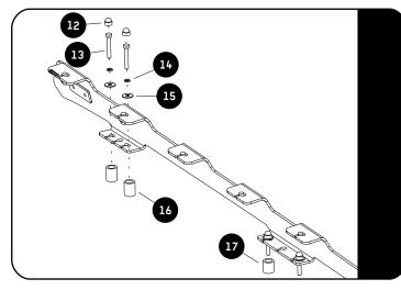
Fit the Foot Rail to the vehicle using M5 x 35 Hex Bolts, M5 Spring Washers and M5 x 13 x 1 Flat Washers (Items 13, 14 & 15) as shown.
