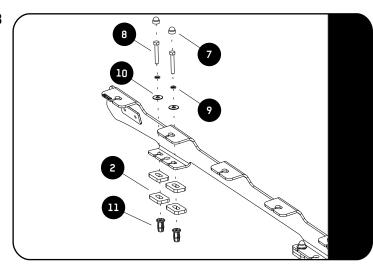
Place a bead of silicone around each of the Jack Nut openings inserted earlier in Step 2.3.
