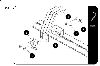
Assemble the Legs (Item 8) to the Leg Mount (Item 3) by using M8 x 30 Button Heads and M8 nyloc Nuts (Items 4 & 7) and the M8 x 20 T-Bolts (Items 1).
