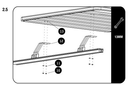
Loosely fit your Slimline II Rack by using M8 x 25 Hex Bolts, M8 x 16 x 1.6SS Flat Washers and M8 Nylocs (Items 10, 11, 13) as shown.
