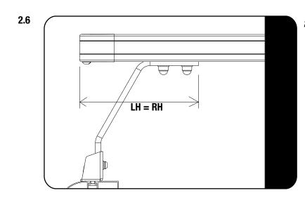
Center the rack on the Legs before fully tightening (LH = RH).
