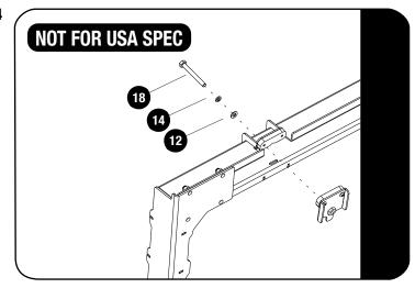
Loosely assemble the Clamps with Spacers to the Rear Side Mount using M8 x 70 Hex Bolts, M8 SS Spring Washers and M8 x 16 x 1.6SS Flat Washers (Items 12, 14 & 18) as shown.
