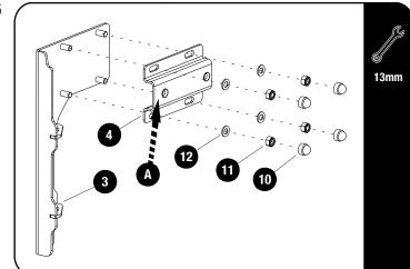
Assemble the Front Support (Item 3) and the Front Side Mount (Item 4) using M8 Nyloc Nuts and M8 x 16 x 1.6SS Flat Washers (Items 11 & 12).
