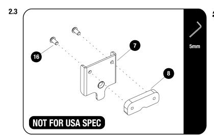
Assemble Spacers (Item 8) to each of the four Clamps (Item 7) using M6 x 12 Button Head Bolts (Item 16).
