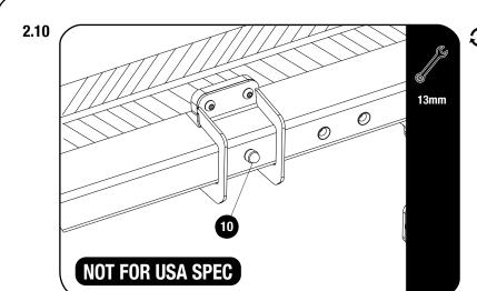
Fully clamp the Side Mount to the top lip of the vehicle's load bin.
