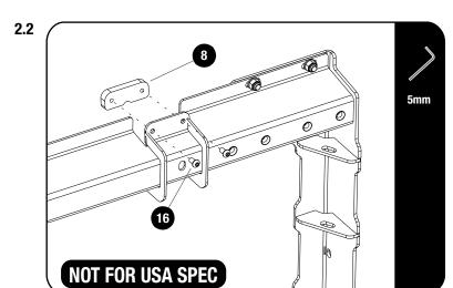
Assemble Spacers (Item 8) to the Rear Side Mount using M6 x 12 Button Head Bolts (Items 16).
