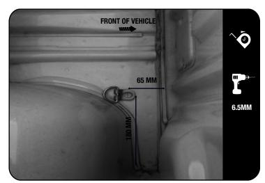
On the front right hand side of the vehicle mark the dimensions as per diagram.
