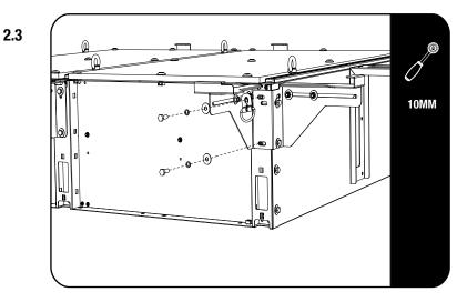
See diagram 2.3 for placement of the D-ring at the rear right side of the drawer. Repeat this step on the left side of the drawer.
