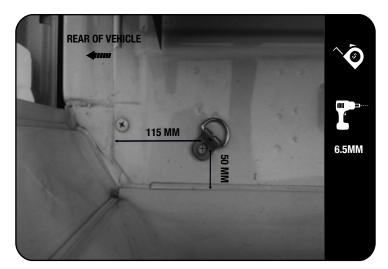
On the rear right side of the load bin mark the dimensions as per diagram.
