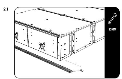
Place the drawer in the vehicle. Fix the track to the drawer. Refer to SSDR010 Fitment Guide.
