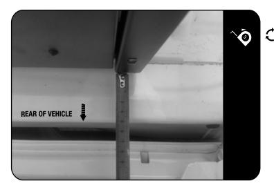
Move the front of the drawer 50mm from the rear of the vehicle and centralize the drawer from left to right.
