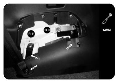
Secure the front and rear tie-down bracket using the existing bolts you removed from the seats and the bottom seat belt bolts. Do this on left and right side of the vehicle.
