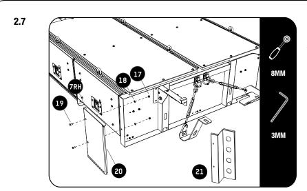
Assemble the two Front Faces (Item 20 or 21) to the Drawer System using M5 x 10 Button Head, M5 Flat Washers and M5 Nyloc Nuts (Item 17, 18 & 19).
