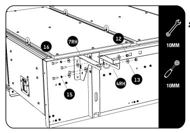
Place the drawer in the vehicle before assembling the wings to the drawer. Refer to 1.1 for wing placement.
