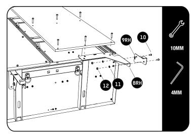
Loosen the rear deck and secure the rear wings as shown. Refer to 1.1 for wing placement.
