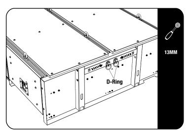
Move the 2 D-rings to the middle mounting holes as shown .
