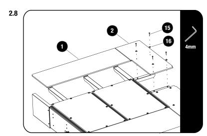
Secure the Rear Deck LH & RH (Items 2 & 3) to the Rear Wing and Rear Support using M6 x 30 Countersink Screws and M6 Finishing Washers (Items 15 & 16) as shown.
