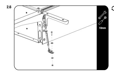
Secure the D-Rings (supplied with SSDR012) in the front of the load bed through the holes drilled in 2.1 using M6 x 20 Hex Bolts, M6 x 19 x 1SS Flat Washers and M6 Nyloc Nuts (supplied with SSDR012) as shown.
