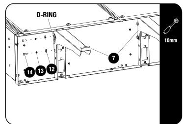
Fit the Front and Middle Side Wings (Item 7) to the drawer using M6 x 16 Hex Bolts, M6 SS Spring Washers and M6 x 19 x 1SS Flat Washers (Items 12, 13 & 14) as shown.
