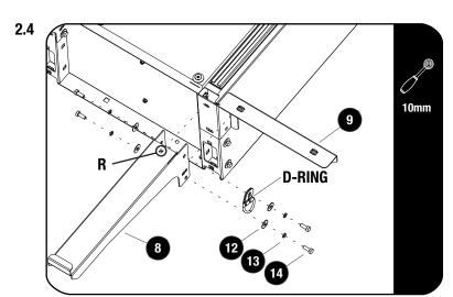
Fit the Rear Wing (Item 9) and the Rear Side Wing (Item 8) using M6 x 16 Hex Bolts, M6 SS Spring Washers and M6 x 19 x 1SS Flat Washers (Items 12, 13 & 14) as shown.
