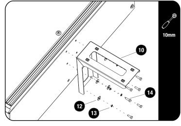
Looking at the rear of the drawer, fit the Rear Support (Item 10) using M6 x 16 Hex Bolts, M6 SS Spring Washers and M6 x 19 x 1 SS Flat Washers (Items 12, 13 & 14) as shown.
