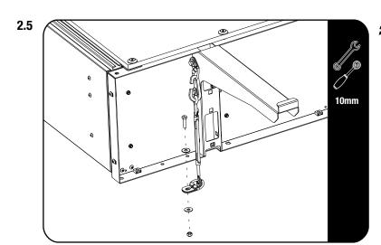
Secure the D-Rings (supplied with SSDR012) in the rear of the load bed through the holes drilled in 2.1 using M6 x 20 Hex Bolts, M6 x 19 x 1SS Flat Washers and M6 Nyloc Nuts (supplied with SSDR012) as shown.
