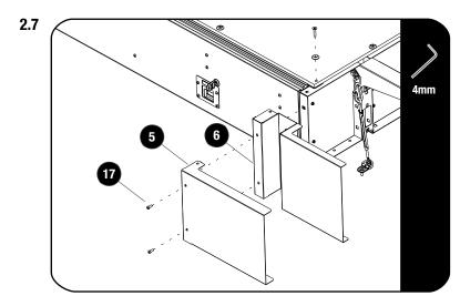
Secure the Front Face Plates (Items 5 or 6) to the drawer using M6 x 16 Button Head Bolts (Item 17) as shown.
